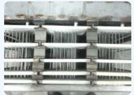
Heater Banks with Straight Wires for High Temperature Hot air generation , Tempering and Glass forming furnaces
